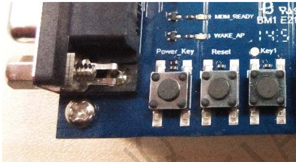
picture 3: power key and reset key
